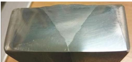
Typical multipass weld-bead placement pattern on the left with one-shot autogenous weld regardless of thickness on the right.
