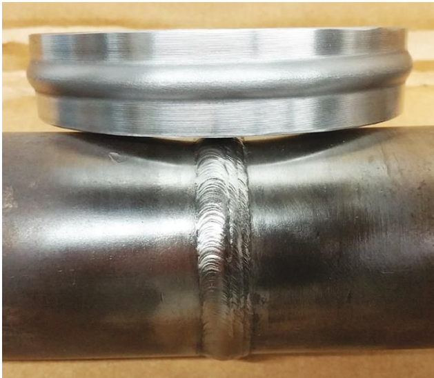
Left: Solid-state fusion or dynamic recrystallization. Right: Inside profile and quality are identical to outside quality.
