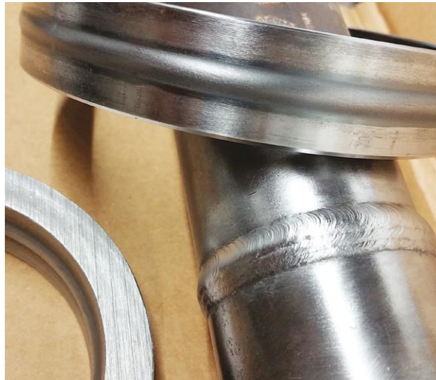
Left: Solid-state fusion or dynamic recrystallization. Right: Inside profile and quality are identical to outside quality.
