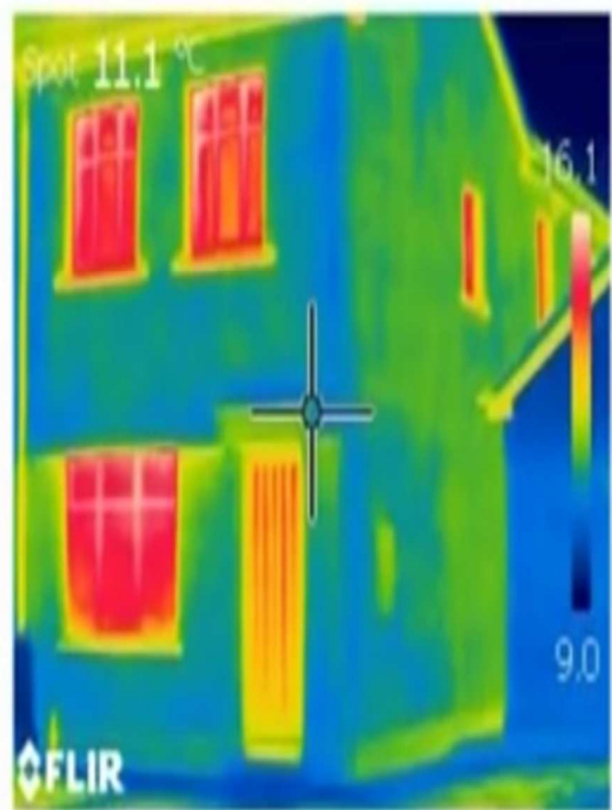
b. After insulation
