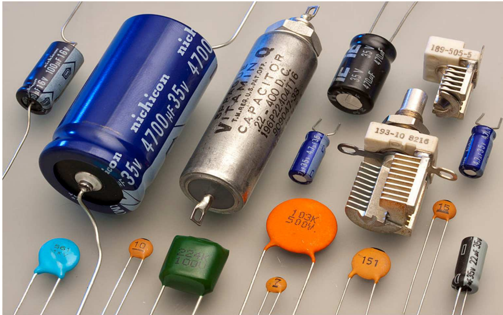
Figure (4.15) Electrical capacitors
