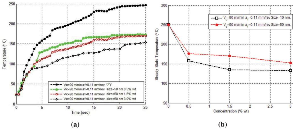
Figure 6. The effect of nanofluid concentration and nanoparticle size on the cutting tool temperature.
