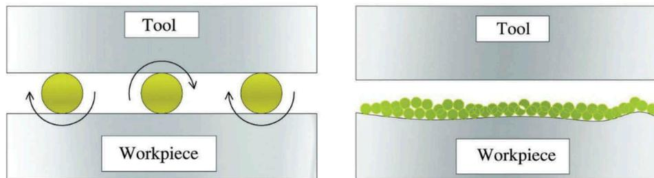
Figure 5. Nanoparticles exhibiting a rolling behavior, thereby reducing the slipping friction.
