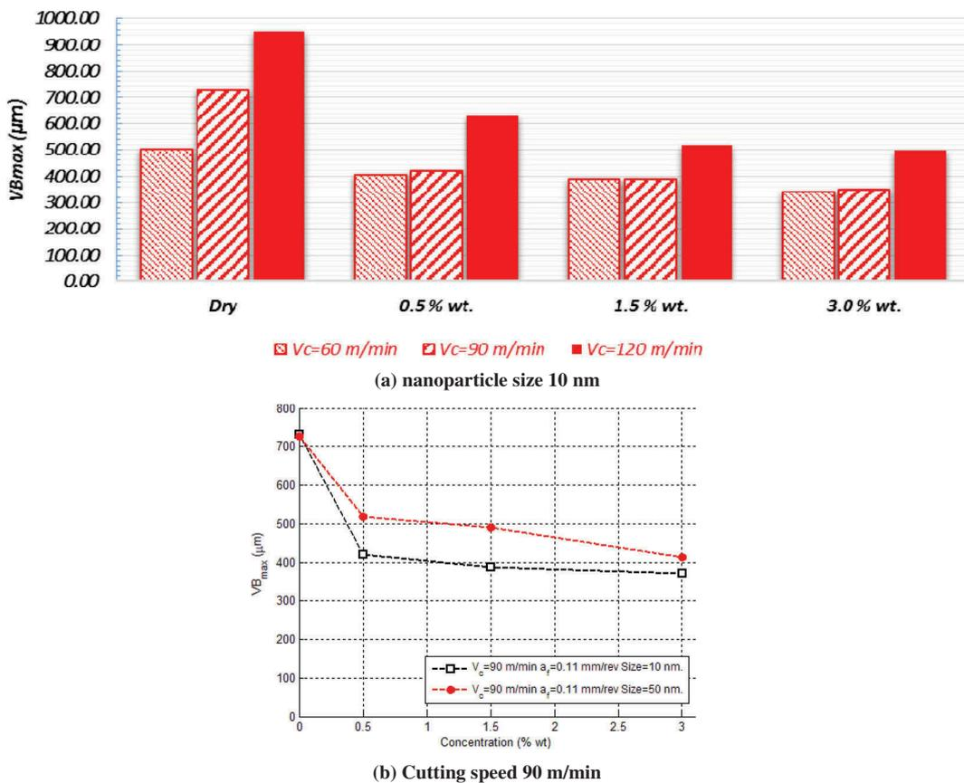
Figure 7. Impacts of nanofluid concentration and nanoparticle size on the flank tool wear (feed: 0.11 mm/rev).
