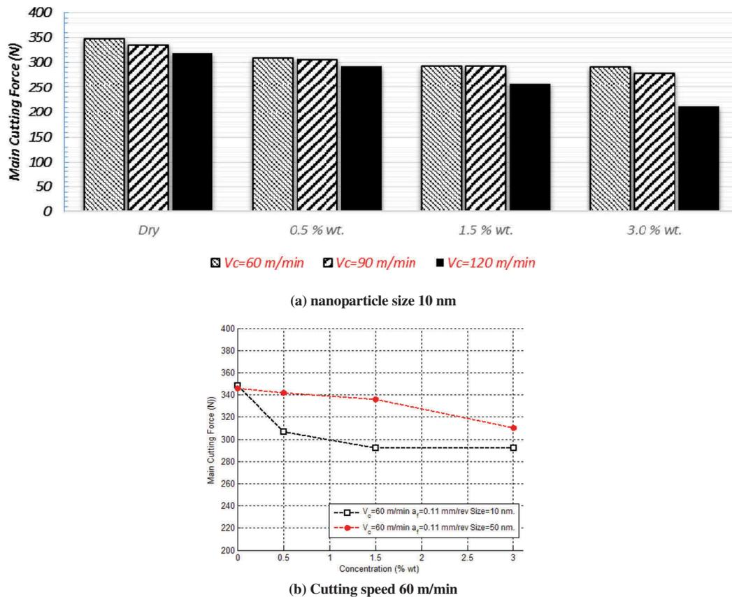
Figure 4. Impacts of nanofluid concentration and nanoparticle size on  $F_c$  (feed: 0.11 mm/rev).
