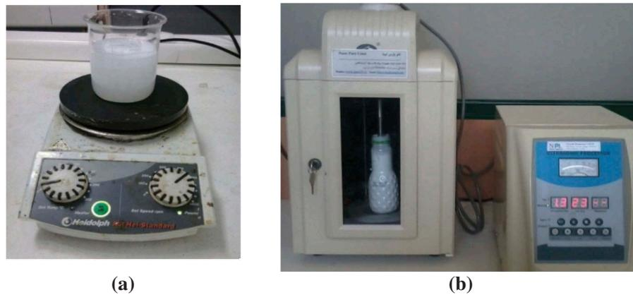
Figure 1. Equipment items used for preparing the nanofluid: (a) magnetic stirrer and (b) ultrasonic stirrer.
