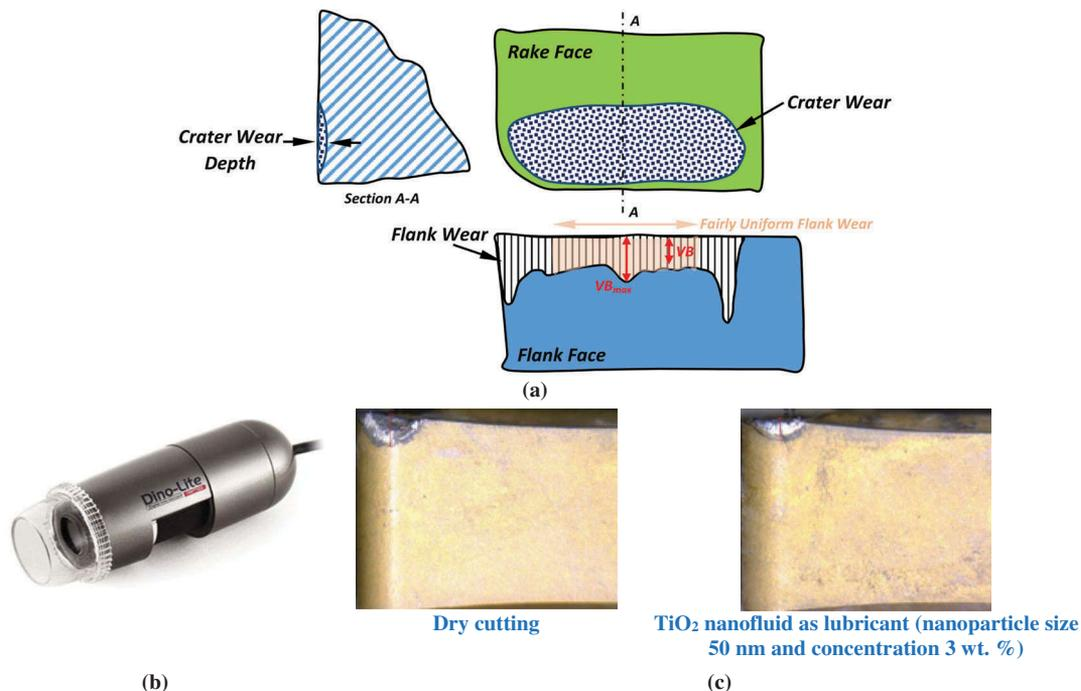
Figure 2. Wear on tool flank: (a) schematic representation, (b) utilized digital microscope, and (c) differences in tool flank wear in case of dry cutting and using  $\text{TiO}_2$  nanofluid ( $a_f = 0.11$  mm/rev,  $V_c = 60$  m/min).
