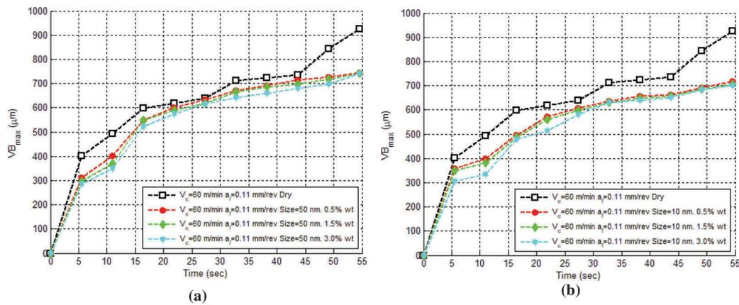
Figure 8. The impact of nanoparticles' size and their concentration on tool wear rate ( $V_c = 60$  m/min and  $a_f = 0.11$  mm/rev).
