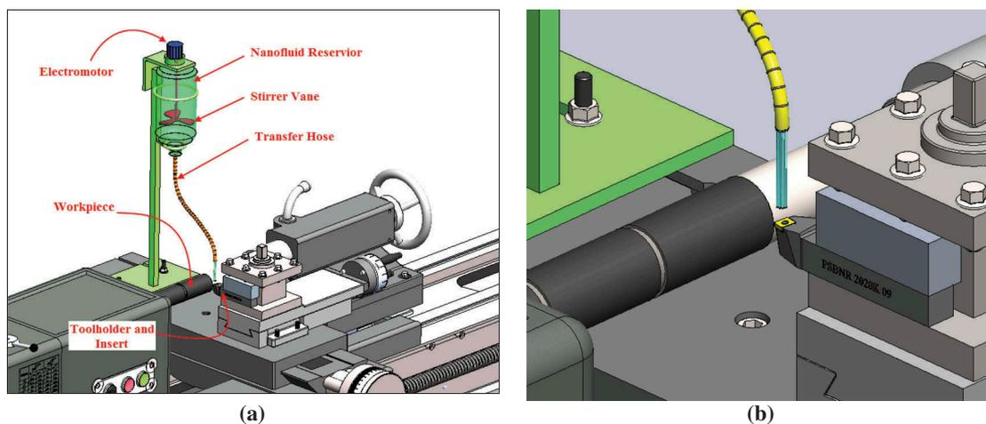
**Figure 3.** The system used to transfer the nanofluid to the machining tool.
